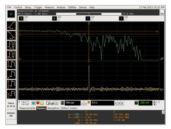
Image 5: FFT of the pulse of the differential math from the calibration edge of the 90000 Q-Series
